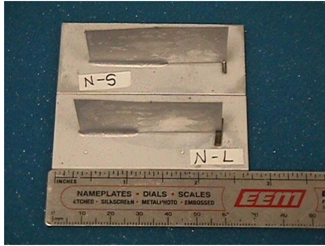
Fig. 32 Photograph of Sample using Flux N Test # 060306, Refer to Fig. 9 Length of fillet N-S: 28.8 mm, N-L: 20.9 mm
