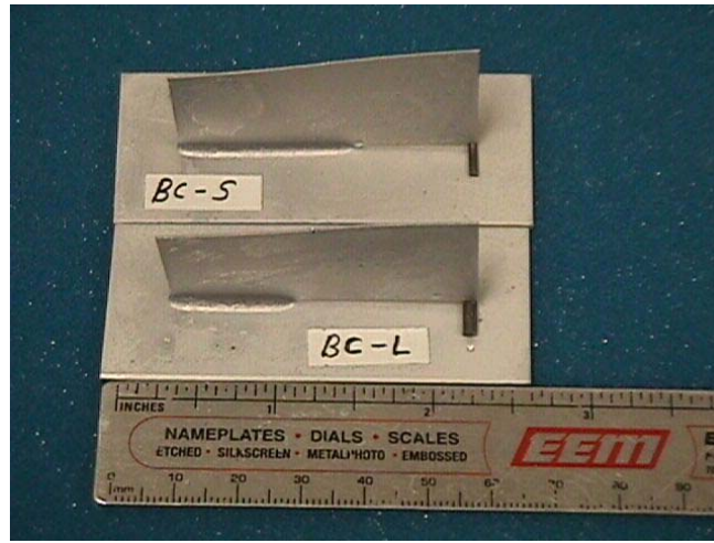
Fig. 29 Photograph of Sample using Flux BC Test # 060206, Refer to Fig. 8 Length of fillet BC-S: 29.7 mm, BC-L: 20.1 mm
