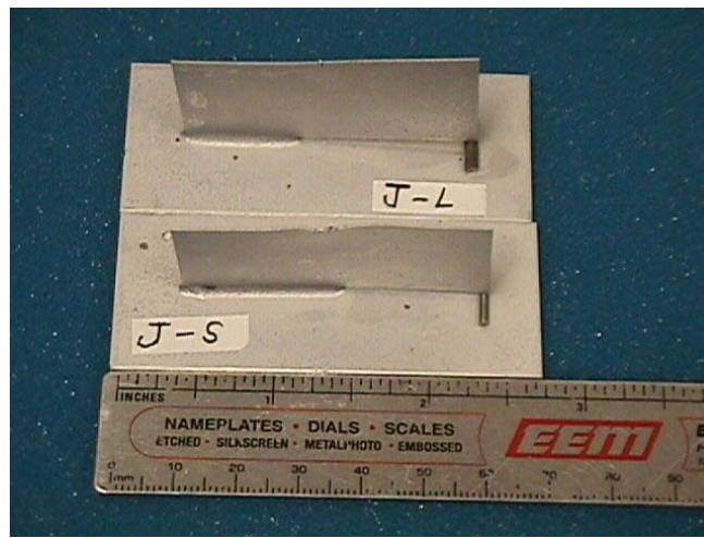
Fig. 31 Photograph of Sample using Flux J Test # 060106, Refer to Fig. 7 Length of fillet J-S: 26.7 mm, J-L: 19.7 mm
