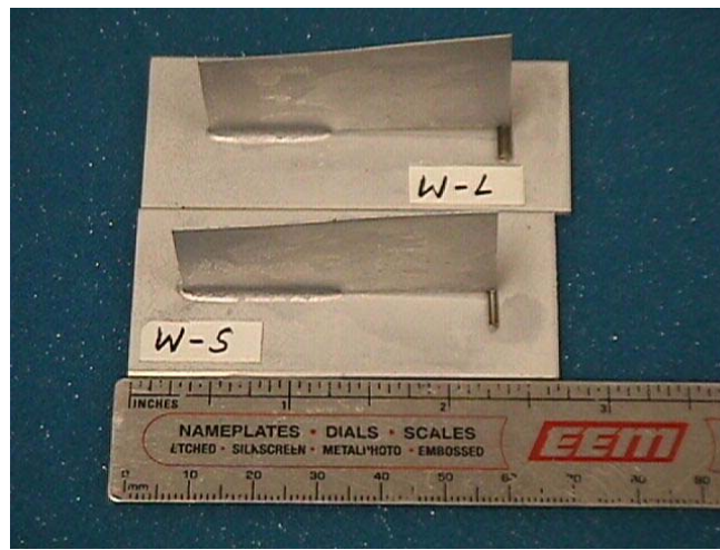
Fig. 35 Photograph of Sample using Flux W Test # 061606, Refer to Fig. 12 Length of fillet W-S: 25.6 mm, W-L: 20.3 mm
