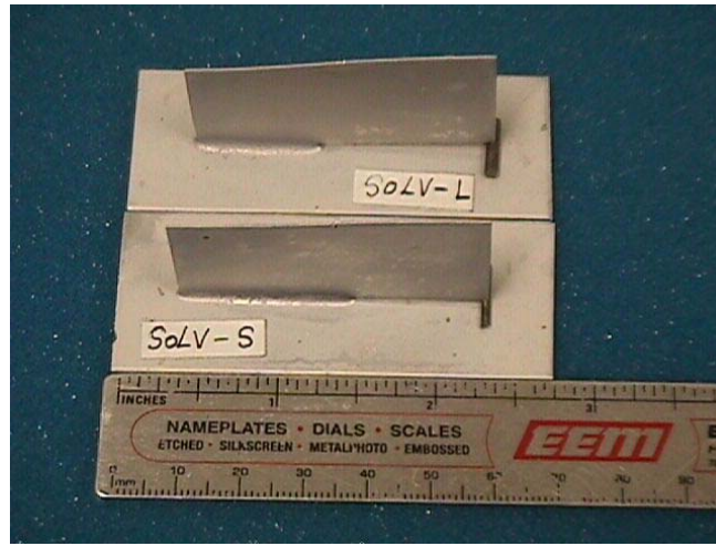
Fig. 34 Photograph of Sample using Flux S Test # 062006, Refer to Fig. 2 Length of fillet S-S: 28.3 mm, S-L: 20.9 mm
