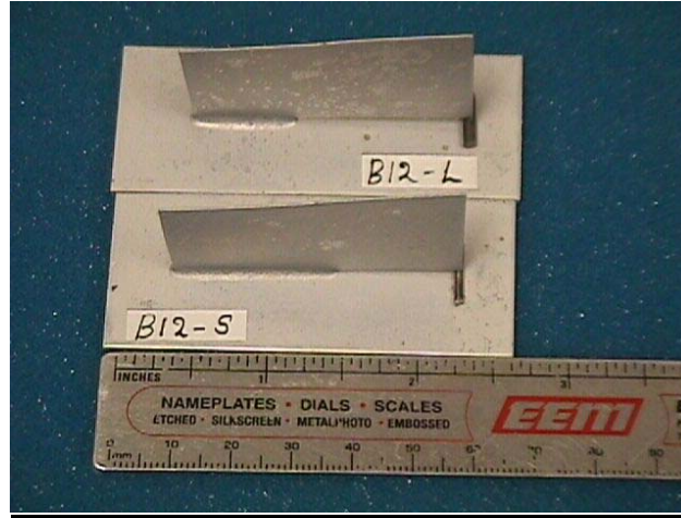
Fig. 28 Photograph of Sample using Flux B12 Test # 061706, Refer to Fig. 13 Length of fillet B12-S: 28 mm, B12-L: 18 mm
